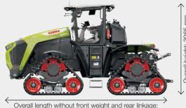
Overall length without front weight and rear linkage: 7350 mm
