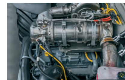
The diesel particulate filter is regenerated automatically.
