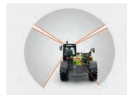
Unobstructed view to the rear thanks to the low-mounted telescopic arm – for safer work.
