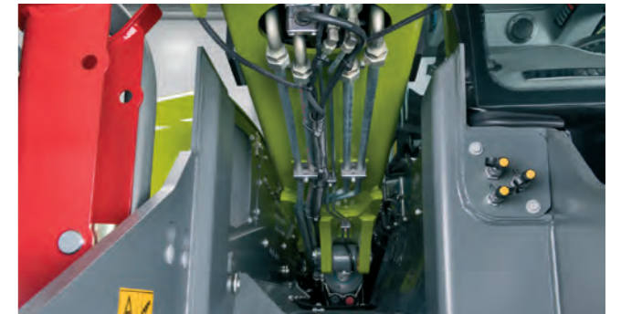
Side telescopic arm guide integrated into the frame as standard with all telehandlers with load capacities above 4,500 kg.
