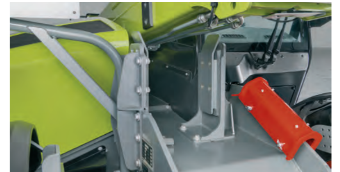
Side telescopic arm guide available for all SCORPION models.
