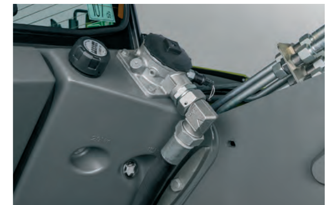
The hydraulic oil level can be conveniently checked via a sight glass. The hydraulic system is protected by a return filter which only needs to be changed after 1,000 operating hours.
