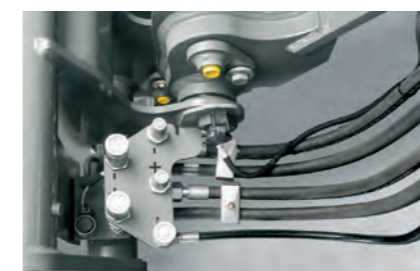
Well-protected hydraulic connections on the implement carrier.
