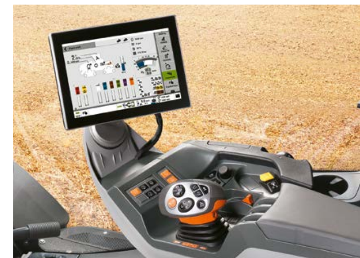
▲ User-friendly operation, intuitive machine settings and unmatched ease of use with the CEBIS on-board information system and CMOTION multifunction control lever.
